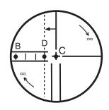
3) Shift the vertical cross-hair line and coincide it with Point D, by revolving the left and right capstan adjustment screws with the adjusting pin. Upon completing the adjustment, repeat the checking operation once more. If Points B and C coincide, further adjustment is not required. Otherwise, repeat the adjustment.
