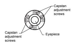
Note: 1 First, loosen the capstan adjustment screw on the side to which the vertical cross-hair line must be moved. Then tighten the adjustment screw on the opposite side by an equal amount which will leave the tension of the adjustment screws unchanged.
