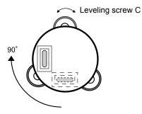
3 Repeat the procedures 1 and 2 for each 90° (100g) rotation of the instrument and check whether the bubble is correctly centered for all four points.
