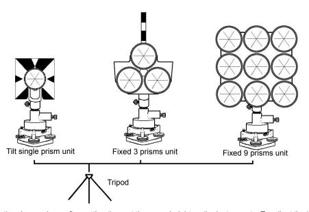
Use the above prisms after setting them at the same height as the instruments. To adjust the height of prism set, change the position of 4 fixing screws.
