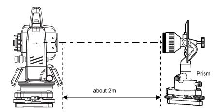
2) Sight through the eyepiece and focus to the prism. Then center the prism on the cross hairs.
