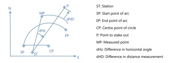
Notably there are four ways available for this application: Stake Out Point, Stake Out Arc, Stake Out Chord and Stake Out Angle.
