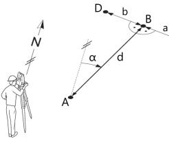
Known: A Known point α Direction from A to B d Distance between A and B a/b Positive or negative offsets
