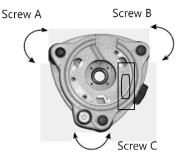
Turn the instrument approximately 90°. Adjust screw C, till the bubble in the center of the level.
