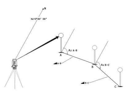
• Radial (A-B, A-C): Measurement is A-B, A-C, A-D, etc.
