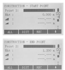
Define start and end points of this construction line in one of the following ways:
