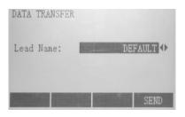
Connect the cable to your computer and select, using the ◀/► keys, the Lead Measure to be output. Press the F4[SEND] key to start transferring data.
