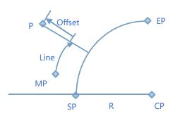
SP: Start point of arcEP: End point of arcCP: Centre point of circleP: Point to stake outMP: Measured point
