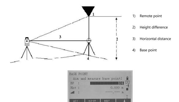
It is possible to measure the height starting from the prism position or from the base point.
