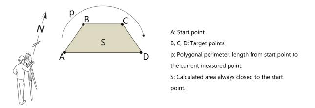
The calculated area is projected onto the horizontal plane (2D) or projected onto the sloped reference plane defined by 3 points (3D). Furthermore, a volume with constant height can be calculated with respect to the area (2D/3D).
