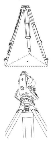
Set up the tripod first: extend the extension legs to suitable lengths and tighten the screws on the midsections. Make sure the legs are spaced at equal intervals and the head is approximately level. Set the tripod so that the head is positioned over the surveying point. Make sure the tripod shoes are firmly fixed in the ground.
