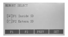
Two methods of memory selecting are available: Inside SD and Extern SD. Select the former using F1 key, the latter using F2 key.
