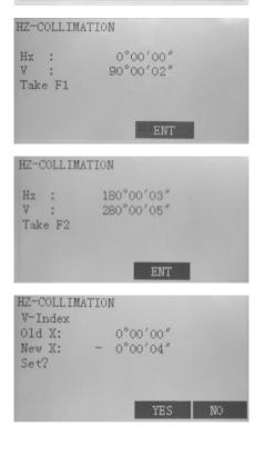
Aim at the cross-hair of collimator at telescope left, and it'll display the horizontal and vertical angles.
