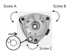
Move the foot screws A and B in opposite direction till the circular bubble is perpendicular to a line shaped with screw A and B. The direction of rotation in left thumb indicates the movement of the circular bubble.
